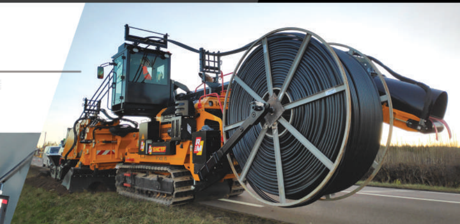
Cable carrier and cable guide on RT400VS with cabin
