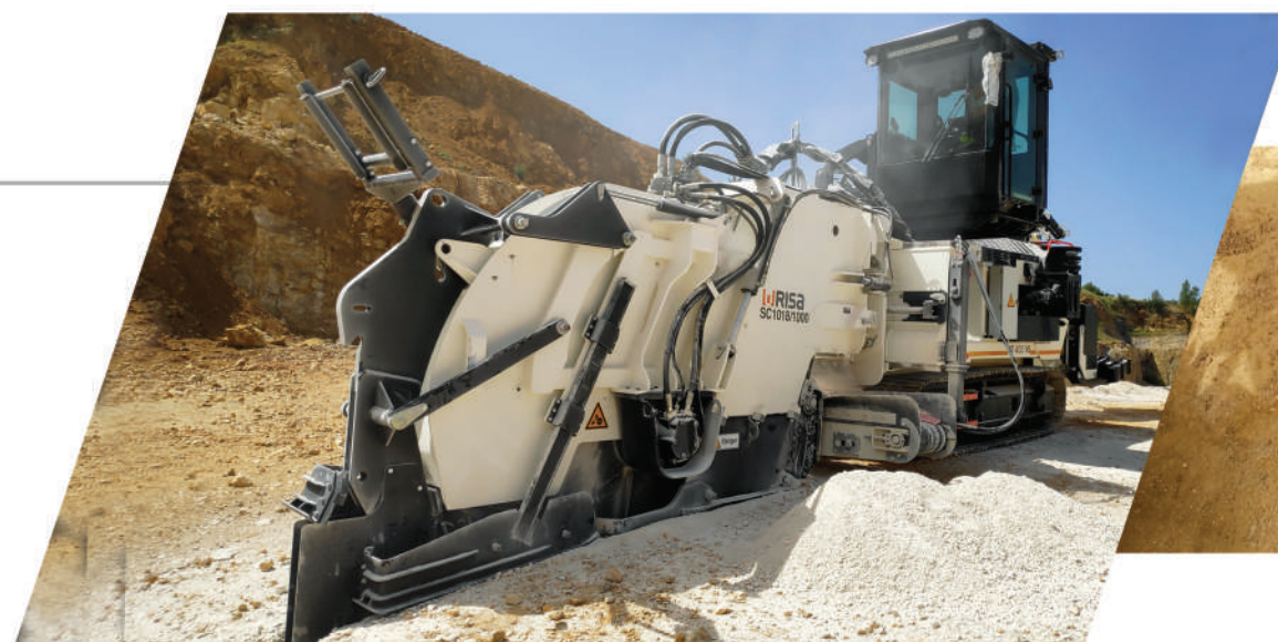
RT400VS with equipment SAW1018/ 1000 and cabin.
