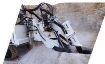
Cable carrier and cable guide on RT400VS with cabin
